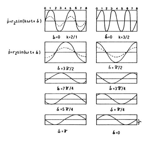
$r_1$ ,  $r_2$  = amplitudes (radius)  $\omega$  = frequency (angular velocity) t = time  $\delta$  = angle of the phase (phase difference)
