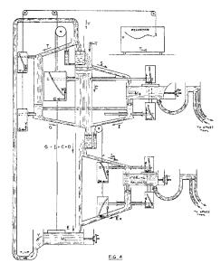
Figure 1: Diagram of one of the hydraulic machines discussed by A. W. Phillips. *Source:* Phillips (1950).
